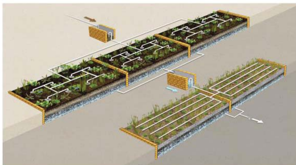
Figure 6: Diagram of a vertical wetland – Traditional French System: Three units in the first stage and two units in the second stage. Source: Sezerino et al. [7].
